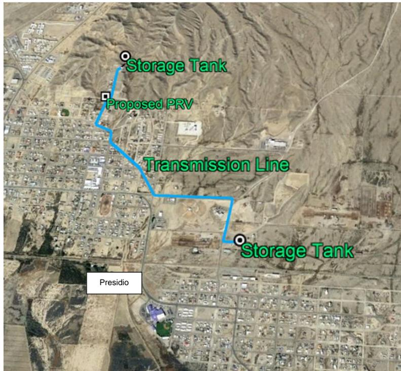
Figure 3 shows the layout of the HWY 67 waterline. This new infrastructure will provide residential and commercial service and will include all standard elements associated with distribution systems such as gate valves, air relief valves, and fire hydrants.
