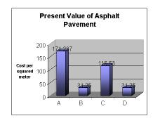
A: Cost of asphalt pavement B: Sealing after 7 years. C: Recarpet at 12 years. D: Sealing at 19 years.
